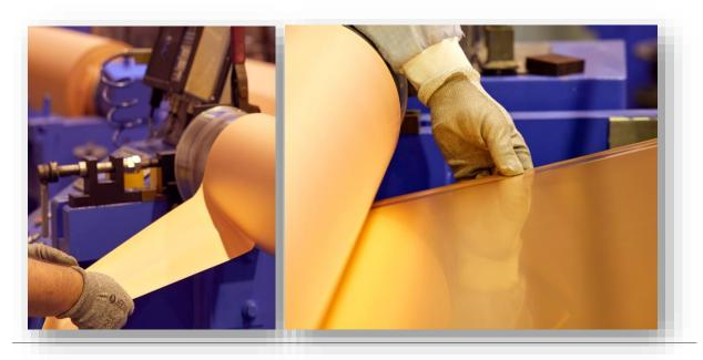
Providing customized solutions with various copper foils ranging from 1.5µm to 200µm
